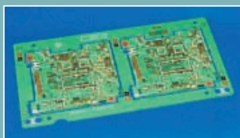
Build-up multilayer PWB (PPBU)
